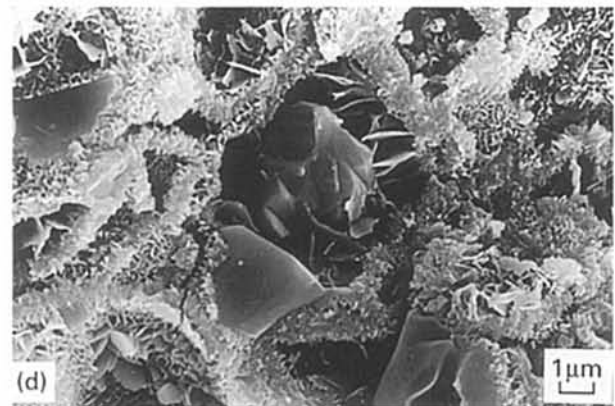
Figure 4 Microstructures of the samples stored at 25°C obtained by SEM: (a) after 24 h of reaction—granules of \alpha -TCP are clearly visible, surrounded by needle-like small apatite crystals; (b) the same sample at higher magnification—a rim of apatite surrounding three \alpha -TCP particles can be observed; (c) after 48 h of reaction—fewer \alpha -TCP granules are visible, and it is possible to observe some bigger plate-like crystals formed in the space originally occupied by \alpha -TCP particles; and (d) the same sample at higher magnification.
